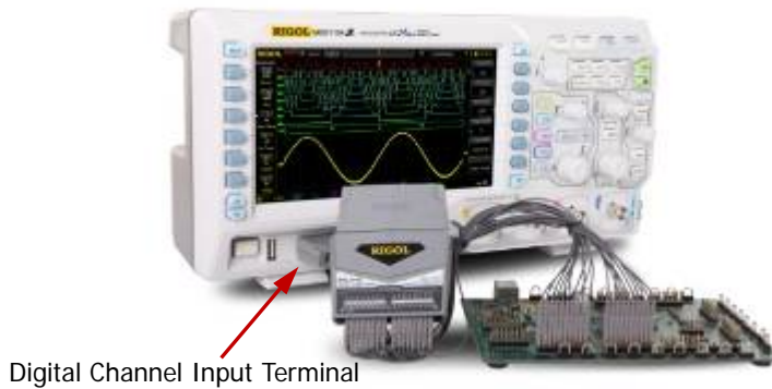
Figure 1-6 To Connect the Logic Probe
